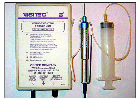
Fig.1: Portable, battery operated vitrectomy machine:tipandhandlecanbere-sterilised.
