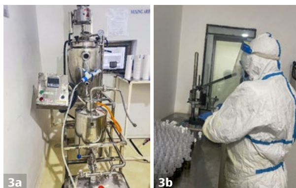
Figure 3 Ruharo Mission Hospital eye drop production facility a. Batch processing unit. b. Manual capping machine.
