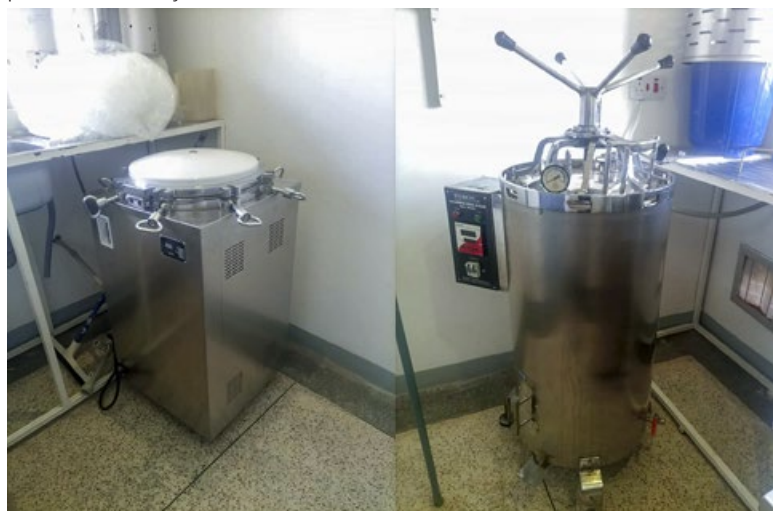
Figure 4 Automated autoclaves used in Ruharo Mission Hospital eye drop production facility.
