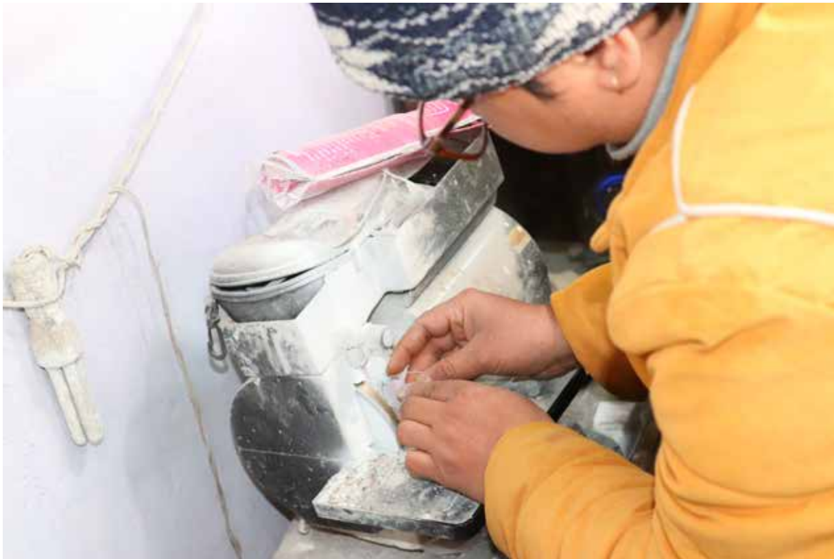
Figure 3 Most opticians in the rural areas rely upon manual edger for spectacle fitting.
