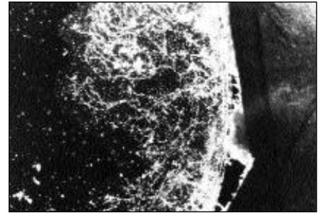
Fig. 2: Grooves etched into a glass surface by organic acids from a mould mycelium (from Kaneko<sup>2</sup>)
