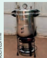
Figure 1: Diagram of a kerosene-burning steam-pressure autoclave
